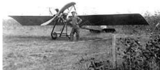
Cessna poses with the monoplane he built during the winter of 1914. It was powered by a 60-hp. Anzani radial engine. By 1915 it had been modified with an improved landing gear, shown here. (Wichita Chamber of Commerce)
