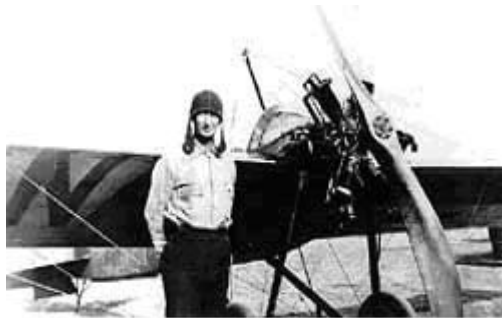
Aviator Cessna strikes a causal pose with the "Comet," a two-place monoplane powered by a 60-hp. Anzani engine. (Smithsonian Institution Neg. # 81-12610)
