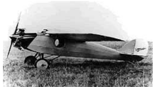
The Cessna "Phantom" with its full cantilever wing was an advanced design for 1927. It was a prototype for the successful "A" series airplanes introduced in 1928. (Stephen J. Hudeck Aeronautical Archives)
